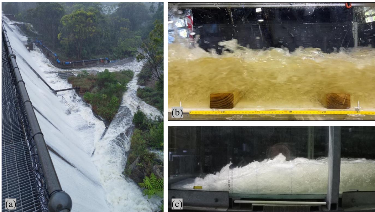
Figure 3. Photos of air-water flow phenomena in field and lab: (a) Air-water flows on spillway of Manly Dam, NSW, Australia in February 2020; (b) side-view of air-water flow processes on spillway (video sequence used for optical flow analysis); (c) side-view of hydraulic jump in the laboratory
