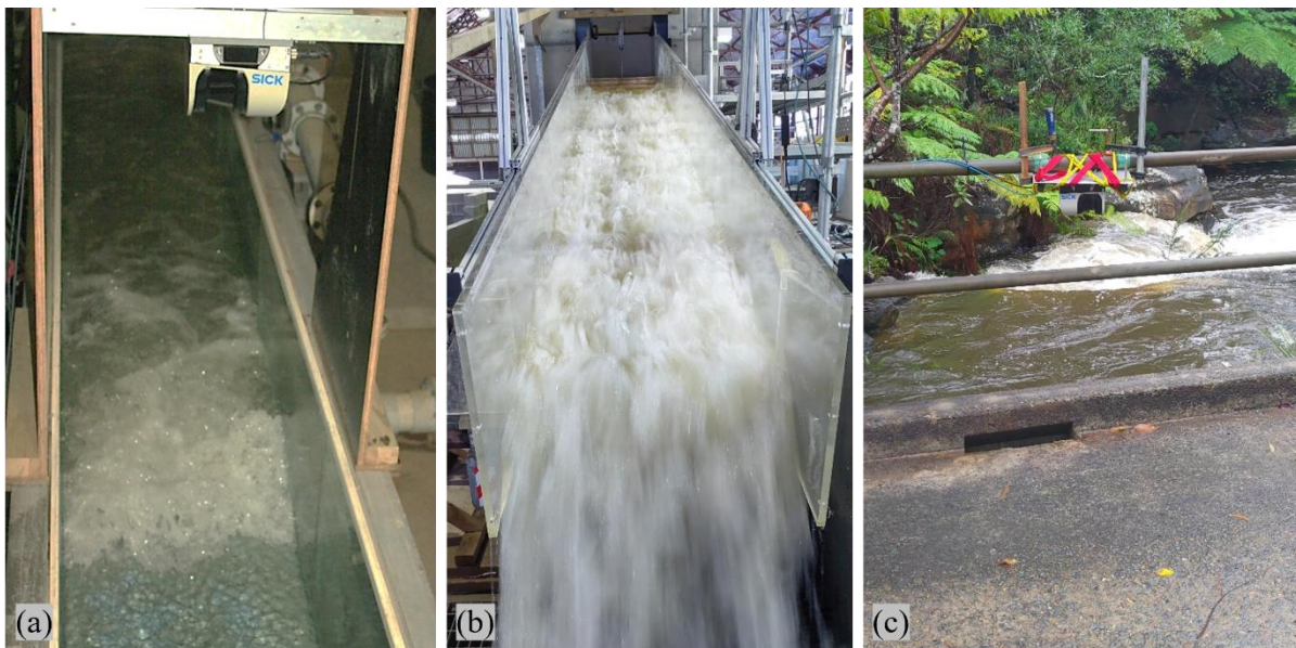
Figure 1. LIDAR measurements of free-surface motions of air-water flows in hydraulic structures engineering at the UNSW Water Research laboratory: (a) fully aerated hydraulic jump; (b) high-velocity air-water flows on a spillway; (c) low-head weir at Manly Creek, NSW.
